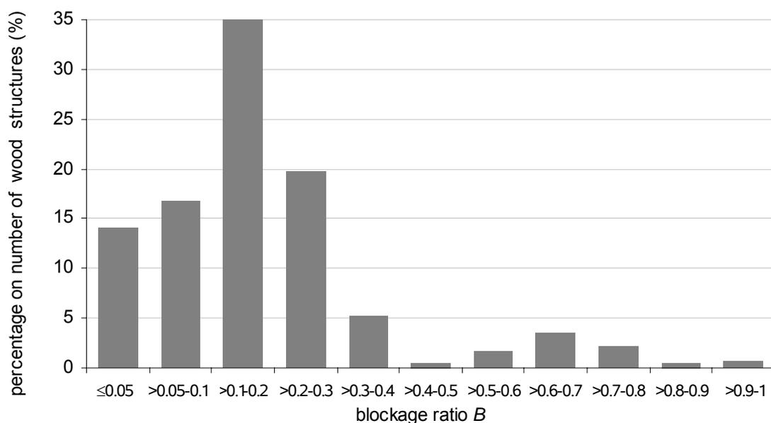
Figure 5.5: Blockage ratio of the wood structures ( $n = 48$  groups of wood structures for which blockage ratio was given separately by the respondents, representing a total number of 400 wood structures).
