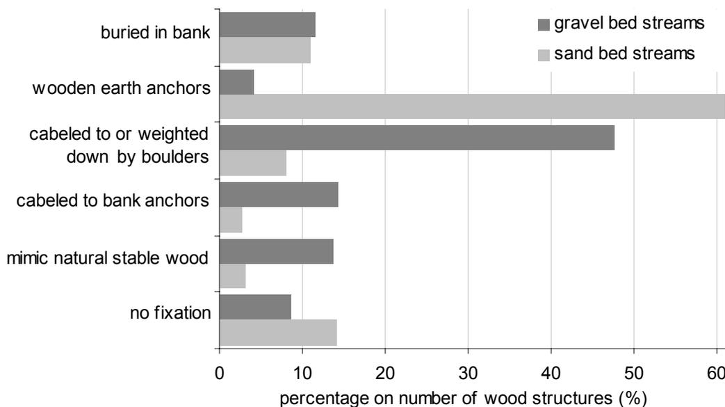
Figure 5.7: Methods used for the fixation of the wood structures in gravel bed and sand bed streams (a total of n = 400 wood structures were considered).
