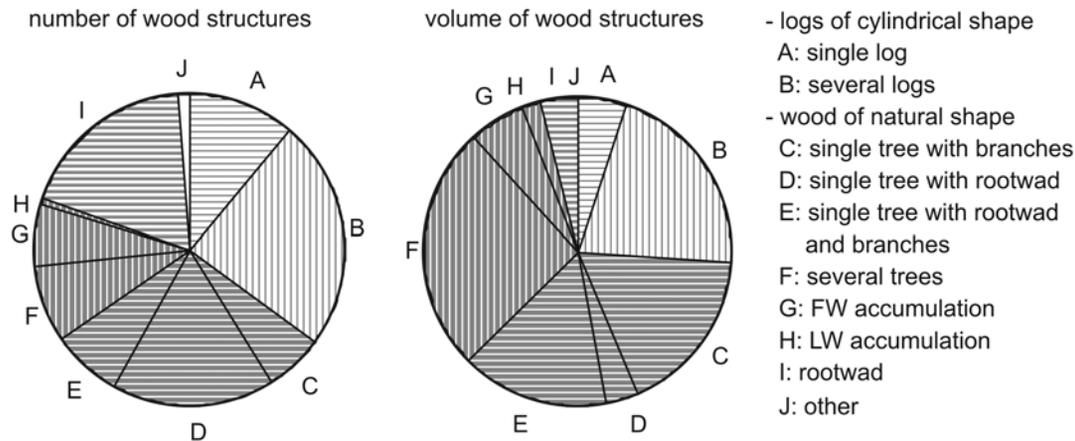
Figure 5.6: Types of wood structures used in the restoration projects related to number and volume. FW = fine wood (diameter approximately < 0.1 m), LW = large wood (diameter approximately > 0.1 m).
